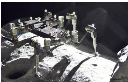
The fully functional SpaceClimber integration-study in the DFKI Robotics Innovation Center Space TestBed
