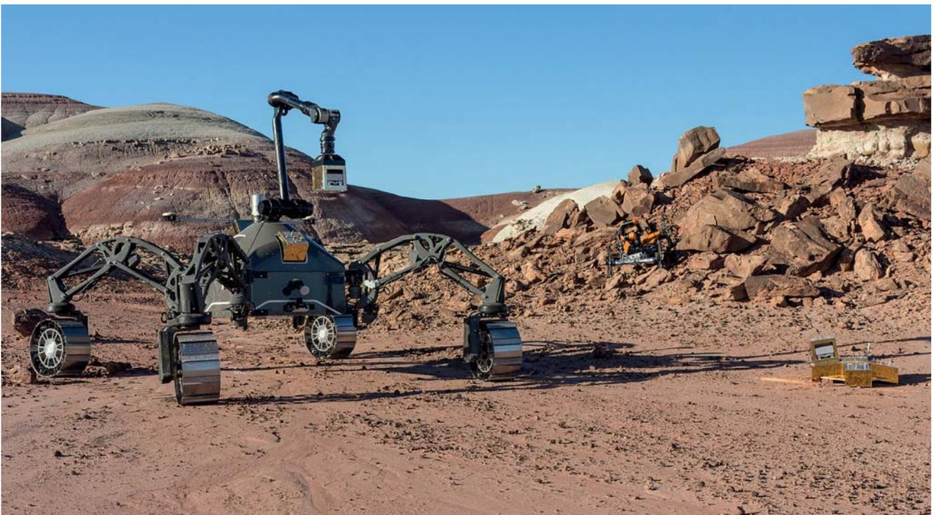
SherpaTT weighs approximately 150 kg and, with its active suspension, is particularly well-suited to explore rough terrain.
