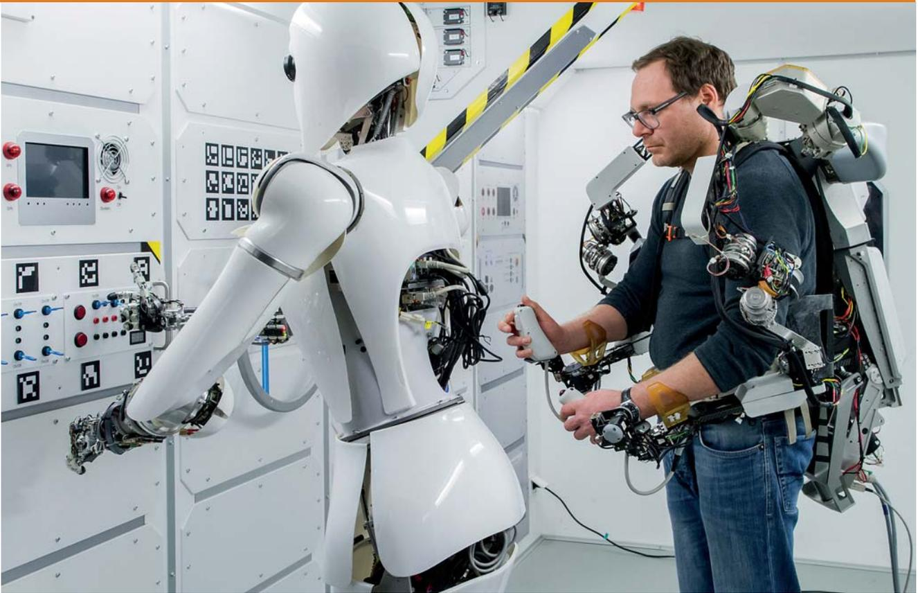
The exoskeleton transmits the movements of the user directly to the robot.
