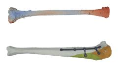
Picking up the 3D model generated in the previous step, a Finite Element Method Simulation is performed, calculating the influence of pressure on the bone-implant structure in terms of stress and strain. While most solutions utilize generic approaches on CPU clusters, this project deploys a specialized FEM approach using Nvidia CUDA that allows for being run on special purpose hardware.
