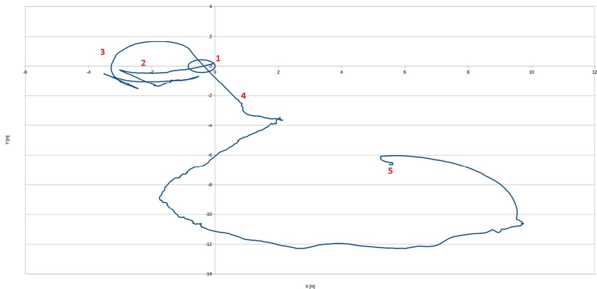
**Fig. 7: Odometry track of the crawler during its deep-sea mission. 1: Descent phase in lander, AHRS records spinning of the lander on cable resulting in ellipse; 2: Backing out of the lander and successful docking; 3: Malfunction of left track visible in odometry, ROV intervention; 4: Attempts to dock; 5: Reboot of control PC**
