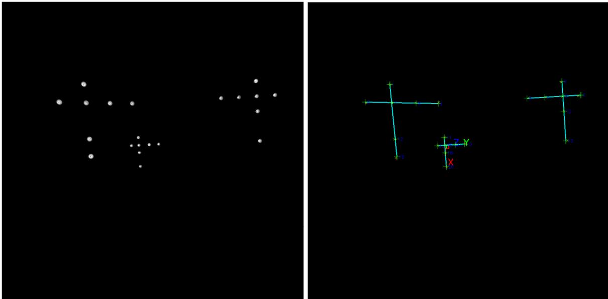
Fig. 5: Left: Camera image taken from the three marker crosses in front of the MANSIO. The exposure control assures a robust view of the LEDs without any disturbing background in the image. Right: Visualization of the marker-cross recognition.
