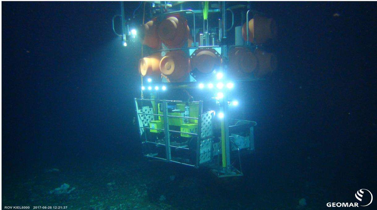
Fig. 3: MANSIO-VIATOR on the seafloor at 1270 m water depth off Svalbard (© GEOMAR).
