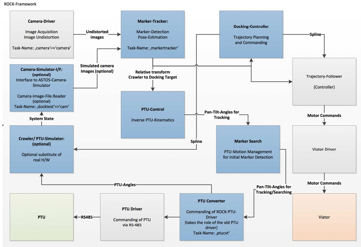
Fig. 4: Block-diagram of VIATOR's docking function.
