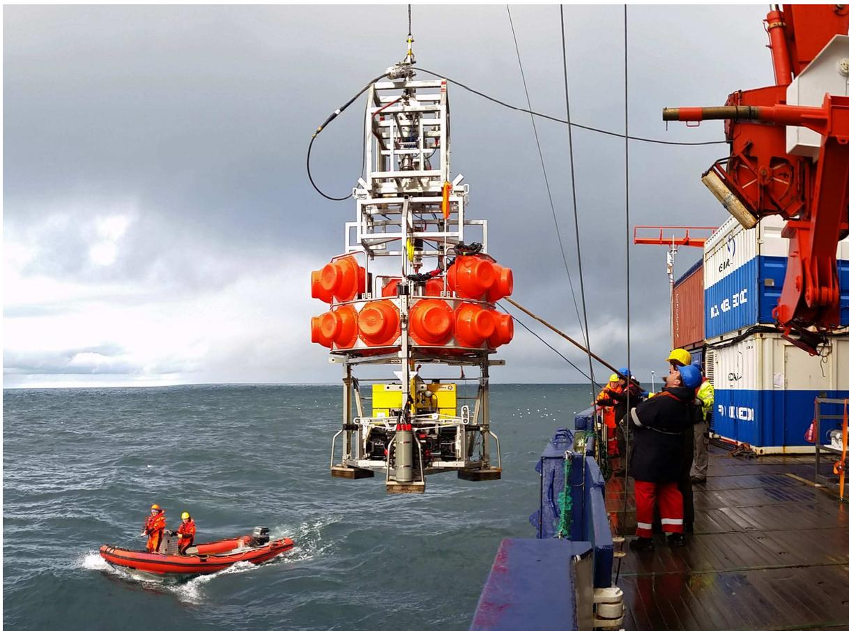
Fig. 2: MANSIO-VIATOR during deployment on Polarstern PS108 (© Lemburg).
