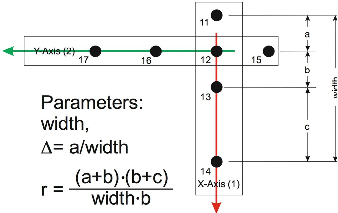
Fig. 5: Coordinate system of a cross-ratio marker-group and definition of marker-group by its cross-ratio parameters width, delta and r (cross-ratio).
