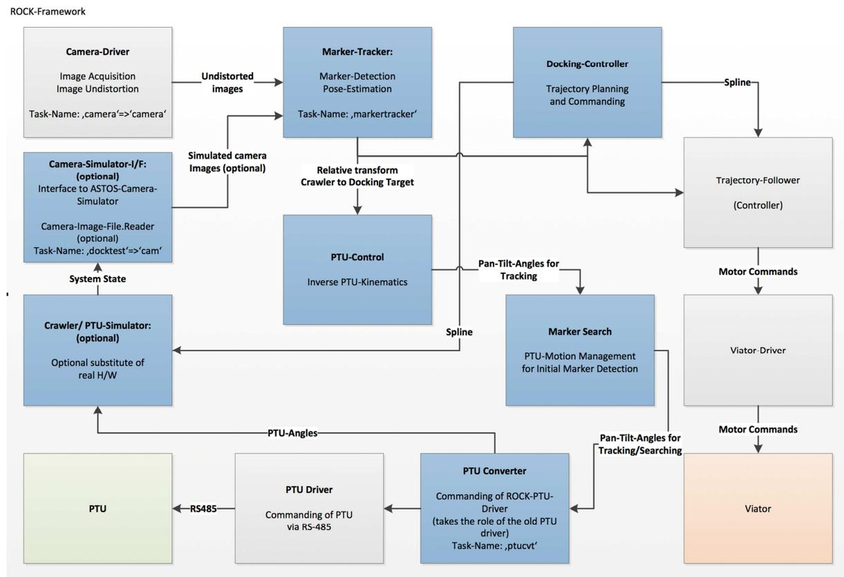
Fig. 4: Block-diagram of VIATOR's docking function.
