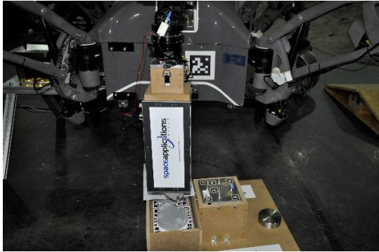
Figure 12 Docking procedure with PBVS (credit: DFKI GmbH 2018)
