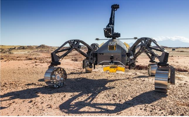
Figure 1: The hybrid wheeled-leg rover SherpaTT during the field test campaign. In the photograph, the system is equipped with modular units used in a multi-robot scenario. The two antennae of the DGPS-system used for ground truth-data can be seen behind the central manipulator.
