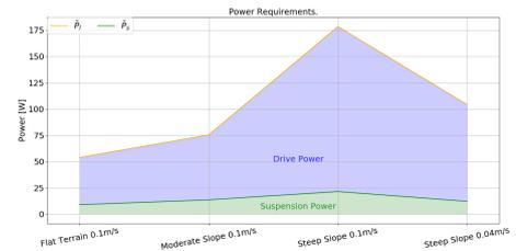
Figure 17: Power for locomotion in different terrains
