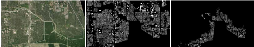
(a) VHR imagery with dataset boundaries (b) OpenStreetMap building footprints (c) Annotated flooded buildings
