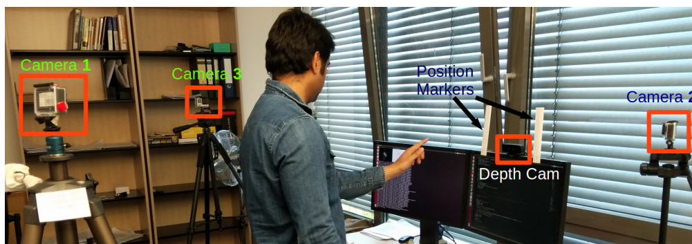
Figure 2. Our setup for in-air signature acquisition. The depth camera is mounted on top of the screen. The position markers on both sides of the depth camera allow capturing of in-air signature within the field of view (FoV) of the camera. Three GoPro cameras are placed around a user to record the hand motion in 3D space from different view points. Camera 3 specifically records the depth variation.
