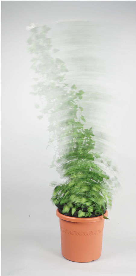
Figure 1: The assembled Overgrown prototype. Using an endoskeleton, a climbing plant can be actuated to, for example, perform a waving motion.
