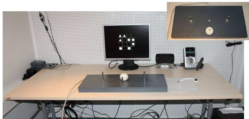
Fig. 1. The experimental set-up and task board for the grasp-to-place task (top view). The task board included two sticks (motor targets) and a sphere which is placed onto a start position as shown in the picture.
