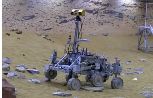
Fig. 2. Testing in the planetary exploration reference scenario: BRIDGET rover in the Marys Yard facility.
