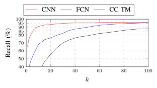
Fig. 4. Objectness ranking results with CNN, FCN, and CC TM objectness. CNN can obtain high recall from 20-40 proposals per image, while FCN requires more to generalize properly. CC TM needs even more proposals to obtain poor recall, which suggests that it is not a good choice for this problem.
