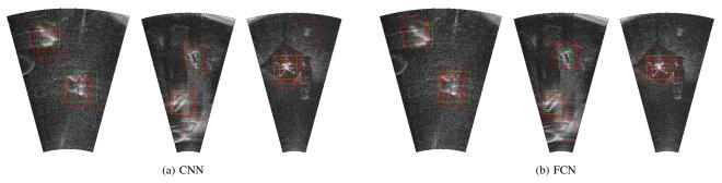
Fig. 7. Sample detections produced by objectness ranking with CNN and FCN scores. We show the top K=10 scoring detections. Red bounding boxes are detections, while green ones are the ground truth. Note how CNN in some cases detects blob objects that are unlabelled in our dataset.
