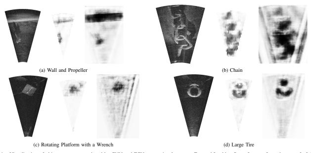
Fig. 6. Visualization of objectness maps produced by CNN and FCN on previously unseen Forward-Looking Sonar Images. In each group: Left is the input image, Center is the CNN objectness map, while Right is the FCN map. Light shades represent low objectness, while Dark ones is high objectness.
