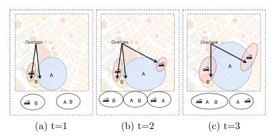
Figure 19: Principle of event relationship, ilustrated as polygon intersection.
