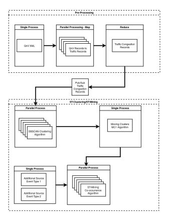
Figure 31: System Architecture.
