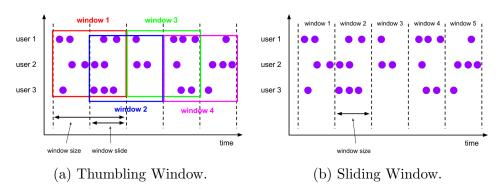
Figure 30: Data Flow Window model.
