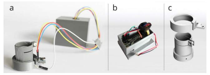
Figure 2. Overview of the measuring device. a) The 3D-printed measuring unit which can be mounted on the water tap. b) The microcontroller in its case. c) The exploded view of the 3D-model.
