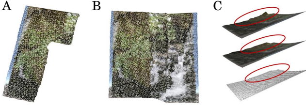
Figure 5. A, B: The completed global surface at frames 350 and 1034. C, top: The completed surface of frame 81 with v = 0.3 and h = 0.1 ; middle: The global surface of frame 81 with v = 0.2 and h = 0.1 ; bottom: The ground truth.
