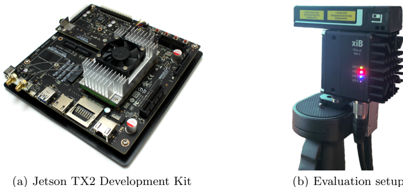
Fig. 4. Our real-time depth estimation is performed on an GPU-based SoC (a). For the evaluation of accuracy we added a reference laser scanner (b).
