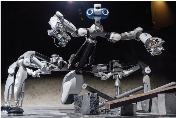
Figure 2. Mantis in erected position by using its front legs for manipulation
