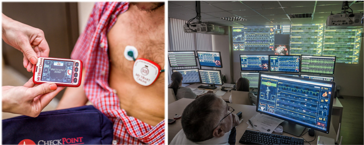
Figure 1: The electrical signals from the interchangeable electrodes connected to the patch (left picture) are removed from a medical device and powered by a battery pack. After filtering the signals, the communication device (left figure) transmits the data to a file server via GSM/Internet. There, data is stored for further processing. After the necessary calculations and transformations, the information is available for visualisation in a telemonitoring centre (right picture).
