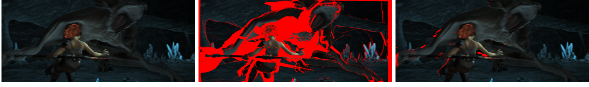
(a) Invisibility Example. Reference image (left), invisibility mask in the dual-frame scenario where no visibility handling is applied (middle), and remaining unmatched areas due to occlusions in the multi-frame scenario where visibility handling is applied (right).
