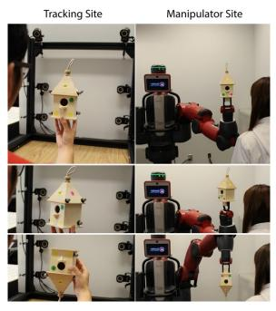
Figure 2: The ReMa system includes a Tracking Site (TS, topleft) and a Manipulator Site (MS, top-right) with bird house object. As the birdhouse is rotated at the TS, the proxy birdhouse at MS is also rotated.
