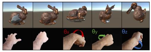
Figure 2: Proprioceptive interaction technique for manipulating virtual proxies (left to right): The user's hand enters the bunny's mesh. By creating a fist, the bunny is selected. Rotations of the fist immediately rotate the bunny.
