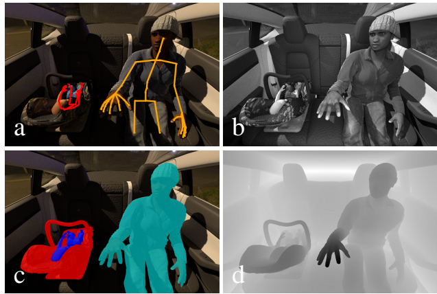
Figure 1. Example scenery of SVIRO together with the provided ground truth data. Left seat: infant seat with an infant. Middle seat: empty. Right seat: adult passenger. a) RGB image with keypoints for human pose estimation. b) Grayscale infrared imitation. c) Position and class based instance segmentation. d) Depth map.
