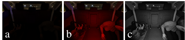
Figure 6. Comparison between a standard RGB image and our simple approach to imitate an active infrared camera system for a dark scenery. a) Standard RGB image in environmental lighting. b) RGB image of the scenery illuminated by an active red light. c) Red channel only of the RGB image of the illuminated scenery (used as infrared imitation in SVIRO).
