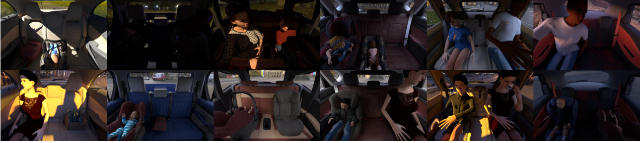
Figure 2. Example sceneries for training (top) and test (bottom) splits for different cars. Each split uses different objects, seats, environments and humans. Some images appear darker, which is why (also in real applications) it is preferred to use an active infrared camera system.
