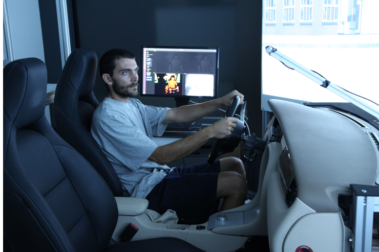
Fig. 1: Driving actions recorded with a 2D/3D camera system mounted above the dashboard. The simulated street scene can be recognized on the right; the computer screen in the background displays the data stream from the camera.
