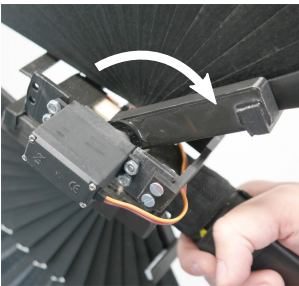
Figure 2: Top: The Drag:on is connected with a long cable to a box holding the microcontroller and circuits. Motor power is provided by an external power adapter. Bottom: A servo motor and connected arm opening a fan.
