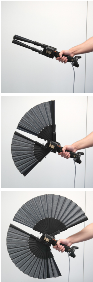
Figure 1: Different states of the Drag:on controller that participants can experience in this demonstration, differing in surface area and weight distribution.
