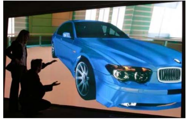
Fig. 5 HEyeWall: High resolution stereoscopic tiled display with 48 beamers (courtesy of Fraunhofer IGD)
