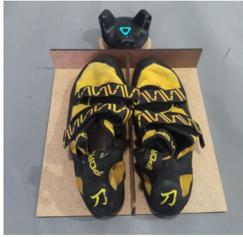
Figure 3: Wooden template to calibrate the climbers feet with the virtual shoe models.
