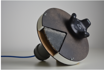
Figure 3: Inspired by a painter's palette, the Haptic Palette is a controller for mixed texture perception in Virtual Reality.
