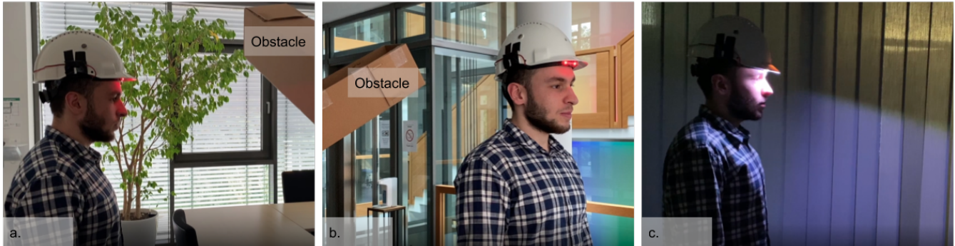
Figure 1: Use case examples: a.b. front and back obstacle warning via directional red LED and scalp haptic feedback. c. automatic flashlight under in dark ambience (the obstacle warning also functions in darkness)
