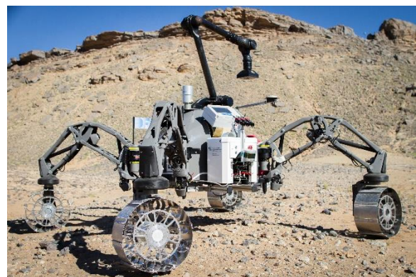
Figure 1 The SherpaTT Rover with the HCRU engineered by DLR Institute of Robotics and Mechatronics mounted during field tests in the desert of Morocco.
