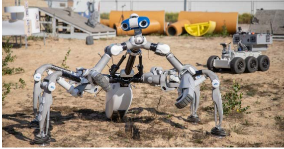
Figure 2: Mantis in manipulation pose during outdoor testing (credit: DFKI GmbH, A. Popp)
