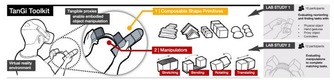
Figure 1: Visual abstract providing an overview of TanGi elements and the context of our two user studies. TanGi consists of *Composable Shape Primitives* allowing the approximation of a variety of objects, and *Manipulators* that provide movable proxy parts.
