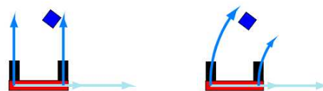
Figure 2: The simulated robot with two out of the four cardinal DoFs (left) and two adaptive DoFs (right)
