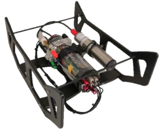
Fig. 2. Sensor-system with the optical FDOM sensor (right) and the sensor tube containing the other sensors (left).
