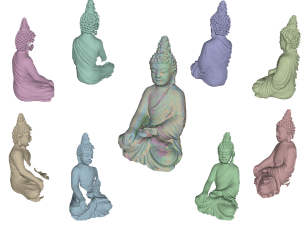
Fig. 1: Partial scans of a full turn and the aligned point cloud (middle).
