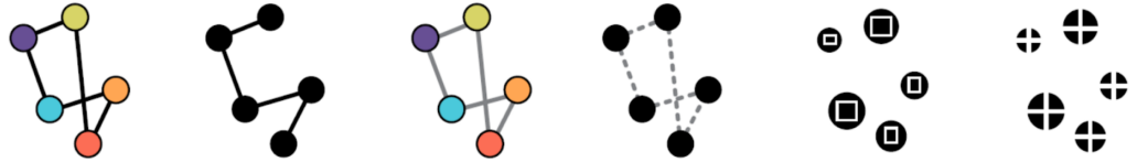
Figure 1 Examples of semantic building fingerprints (SBF). With topology (1-4): semantic spatial graph, through-path-graph, semantic connection graph, spatial distance. Without topology (5, 6): envelope area, center of room.
