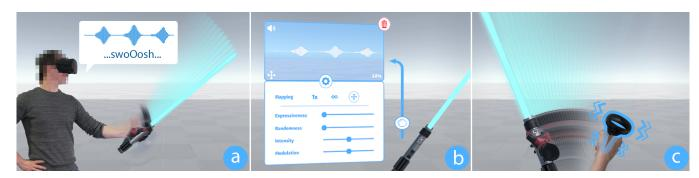
Figure 1: With the Weirding Haptics design tool, one can design vibrotactile feedback in a virtual environment using their voice. a) A designer waves a lightsaber in the air while vocalizing the intended feedback. b) A *vocalization layer* depicts properties of the tactile experience and allows for switching mappings as well as fine-tuning using modifiers (sliders) directly in VR. c) While waving the lightsaber, the vibrotactile feedback can be felt with the VR controller.
