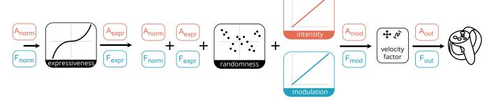
Figure 7: The playback pipeline. Based on the normalized samples produced by the mapping used, we first compute the *expressiveness*, then add the *randomness*, and later apply the *intensity* and *modulation* respectively. The resulting features are multiplied by the relative velocity of the user's movement for motion or positional mappings.
