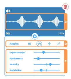
Figure 4: Graphical representation of a vocalization layer. a) The *vocalization* is represented as a stylized waveform. b) The designer can switch between different *spatio-temporal mappings* to try out different experiences, c) or fine-tune the experience by manipulating the *modifiers* using sliders.
