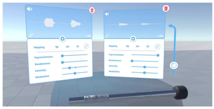
(a) Design of vibrotactile feedback for a slider with textures on top. Here, the difference in vocalization strength (see waveform) is balanced out using the expressiveness and intensity modifiers
