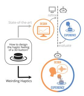
Figure 2: To design the tactile experience of a virtual 3D button, state-of-the-art design tools require designers to go back and forth between designing low-level parameters on a desktop computer and experiencing tactile feedback in VR. In contrast, Weirding Haptics enables designing *inside* the VR environment through vocalizations and supports fast-prototyping through a rapid iterative process.
