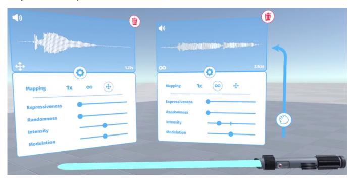
(b) Design of vibrotactile feedback for a virtual lightsaber. Here, a layer with a continuous mapping provides active background vibrations, while a layer using a motion mapping emphasizes the swing of the lightsaber.
