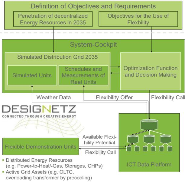
Fig. 1 Interconnections and objectives of the DESIGNETZ project [15]
