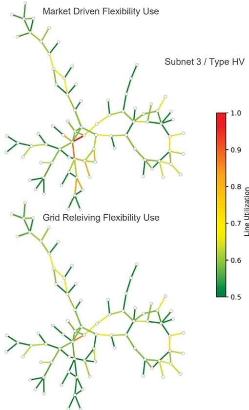
Fig. 6. Line utilization for exemplary 110kV distribution grid, before grid-relieving flexibility use (top) and after (bottom)
