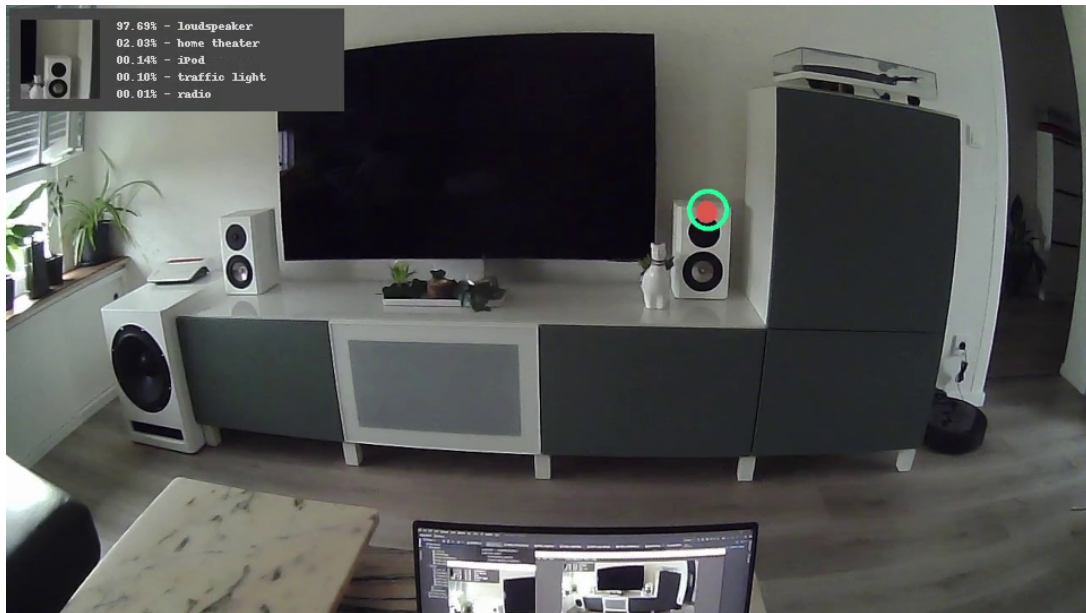
Fig. 4. Screenshot of the visualization sink of our sample application. The user’s recent gaze (red dot) and fixation point (green circle) are on a loudspeaker, which is the top-1 prediction for the corresponding image patch (upper left).
