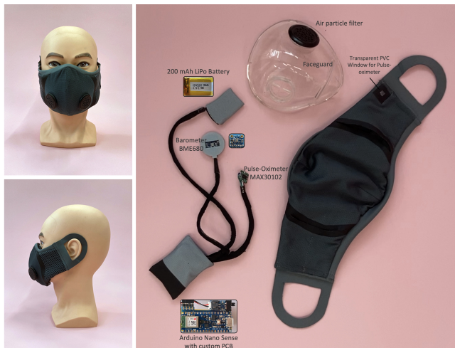
Figure 6: Image of current prototype of the smart mask
