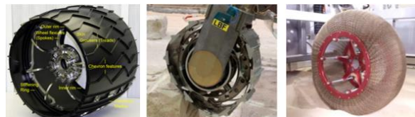
Figure 13: Different wheel types: (left) rigid, (center) deformable and (right) spring tire.
