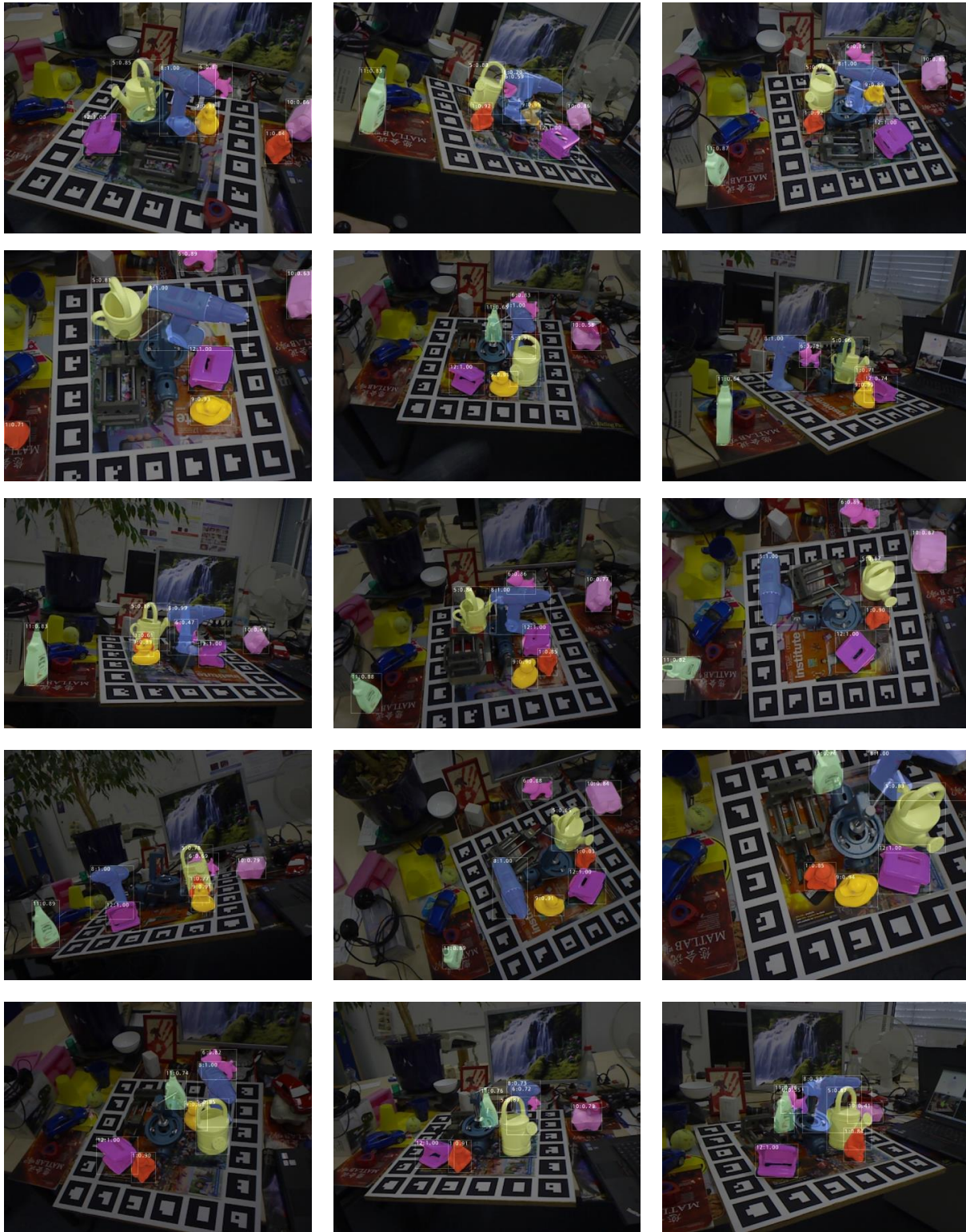
Figure 5. Qualitative Results on LM-O [5]: We render the objects with estimated pose on top of the original images. The presented confidence score are from the 2D object detection with FCOS detector [63].
