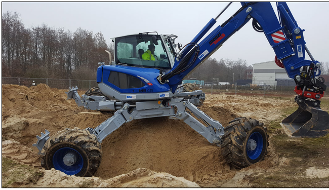
Fig. 1. DFKI's walking excavator (photo by Felix Bernhard).
