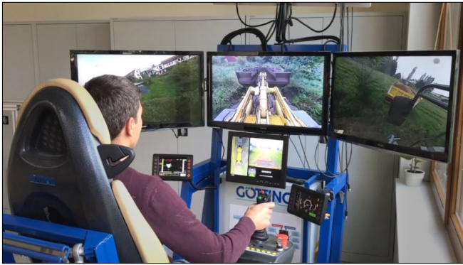
Fig. 5. Control station for teleoperated heavy machinery (Götting KG).
