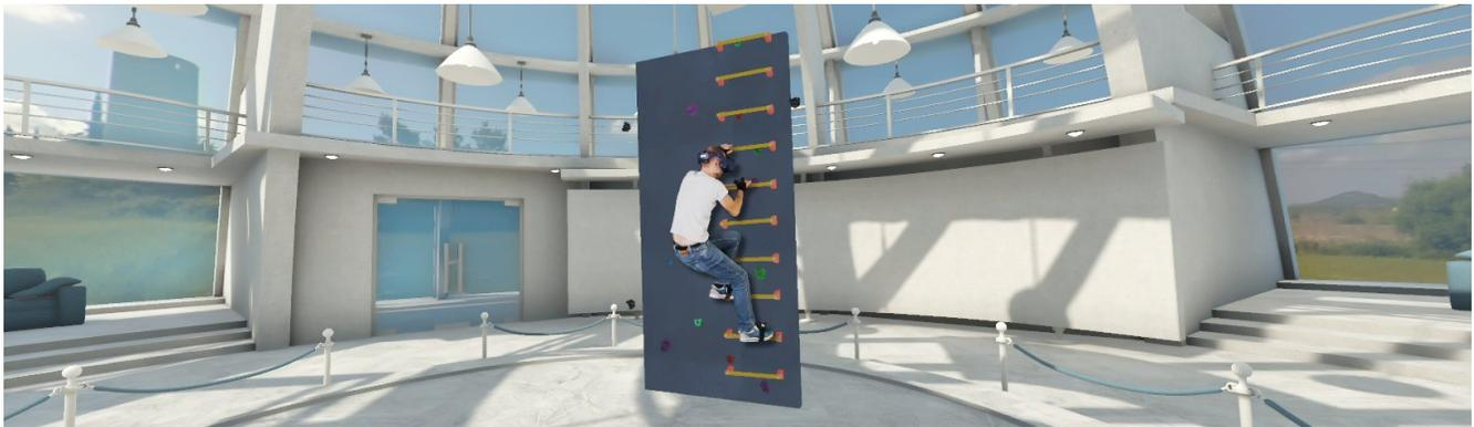
**Figure 1: Virtual Reality rock climbing on a physical climbing treadmill. This allows for continuous climbing while wearing a head-mounted display. With the system presented in this work, we implemented different virtual scenarios. In this showcase application, the climber is placed into a virtual showroom.**
