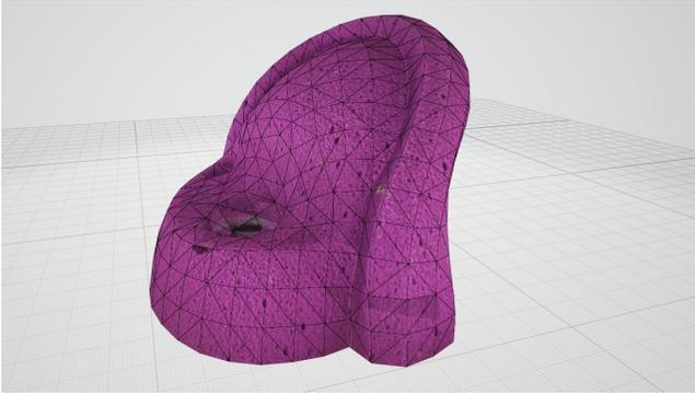
**Figure 5: Having exact representations of the climbing holds helps to establish a strong and precise grip on the first try. The number of polygons of the models had to be reduced to give a smooth, high FPS experience during climbing in VR.**
