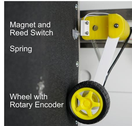
**Figure 3: We designed a spring loaded arm that presses a wheel onto the belt of the climbing wall. A rotary encoder mounted to the wheel measures the rotation while a reed switch detects the start of a new revolution of the belt by means of a single magnet glued to the belt.**
