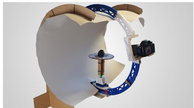
**Figure 4: We used an open source photogrammetry rig that allows one to take a set of pictures from an object from different angles. These pictures were used in Meshroom to reconstruct 3D models of the climbing holds.**
