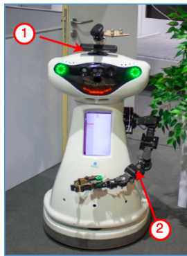
Fig. 2: MBot: 1) Head camera used in this project 2) Robot manipulator used in the experimental part of this work
