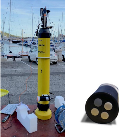
Figure 1: Argo APEX platform with attached sensors, including
