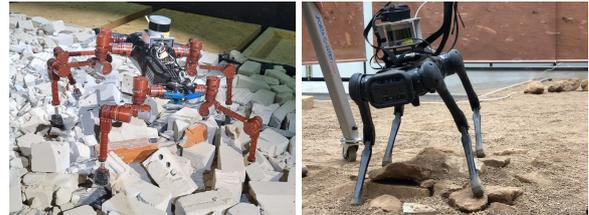
(a) CREX walking over a rubble field (b) Aliengo inside the Mars Terrain Simulator of ALTEC
