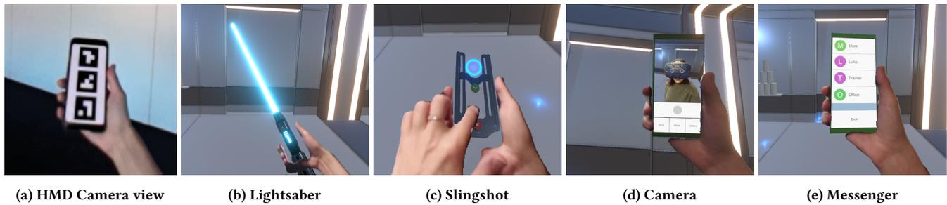
**Figure 3: A smartphone is tracked using on-screen markers in (a) and represented in VR as (b) a lightsaber, (c) a catapult with haptic feedback, (d) an in-VR digital camera, and (e) a simulated messaging application.**
