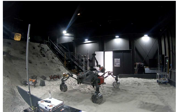
(a) Loose Sand Tests
