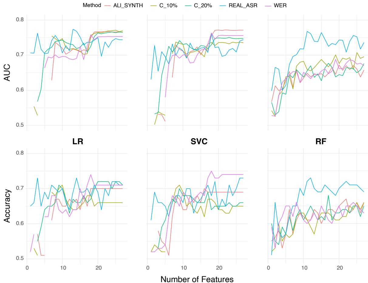
Figure 1: Visualization of results from the machine learning experiments. The number of features used to train the model is represented on x-axis. Logistic Regression(LR), Support Vector Machine(SVC), Random Forest(RF). Area Under Curve (AUC).
