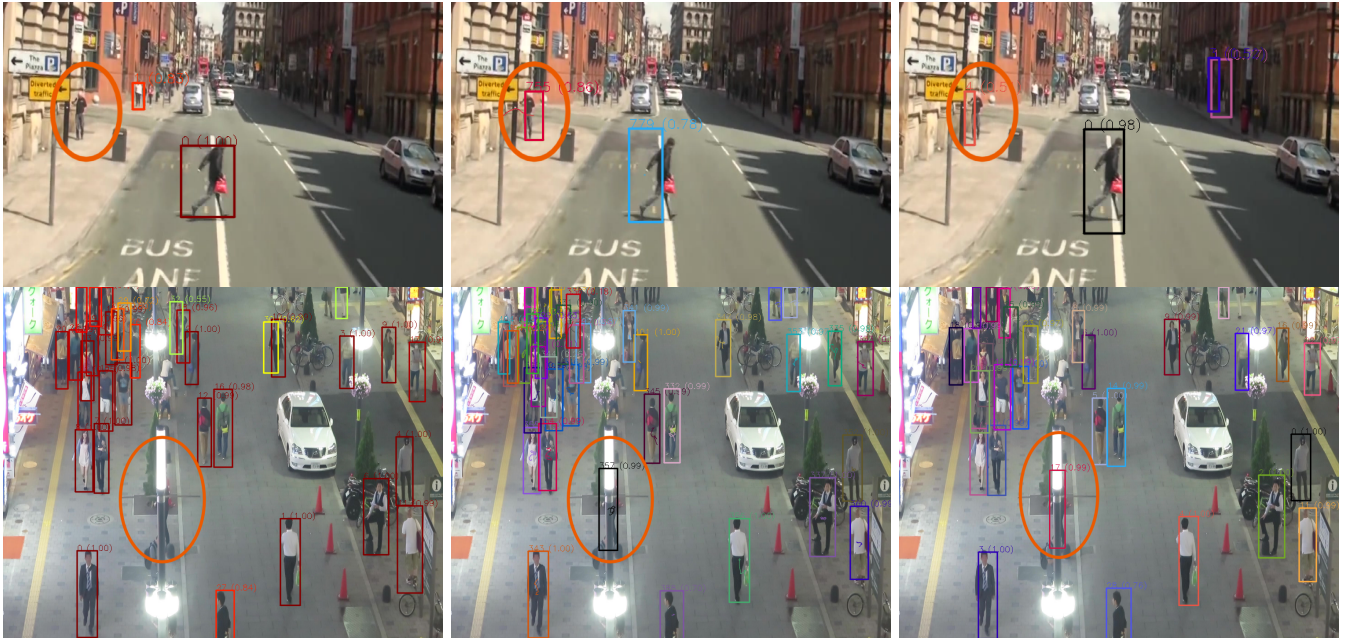
Fig. 5. Qualitative comparison of Faster-RCNN (left), Integrated Object Permanence (IOP) with particles (center) and IOP lite (right). The highlighted persons are hard to detect but can be recovered by using spatio-temporal information at inference time without sequential training data.
